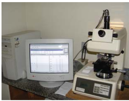
FIGURA 2 – Microdurômetro (shimadzu micro hardness tester hmv - 2000 / Shimadzu Corporation – Kyoto, Japan)
